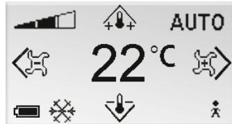
Figur 5. Main view in the display of the room unit.
