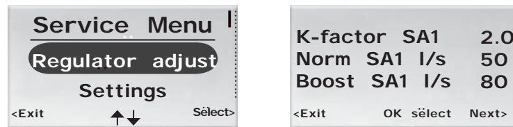
Figur 6. Image for selecting Regulator adjustment settings and view for setting the K-factor and the damper for supply air in air duct 1.
