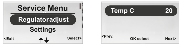
Figur 8. Image for selecting Regulator adjustment settings and image for setting the existing room temperature.
