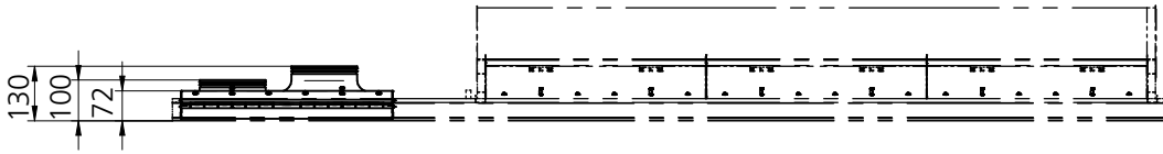
Figure 65. PACIFIC SA/EA, view from side and with capacity module in right-hand version.
