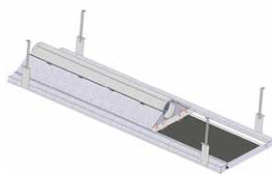
Figure 53. Example of beam suspension with mounting strips.
