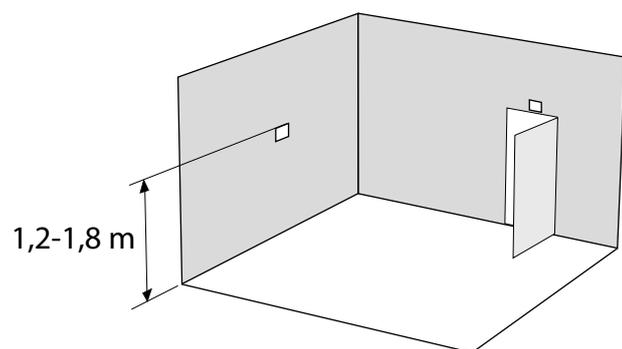
Figure 1. Placement of WISE OCS on the wall.
