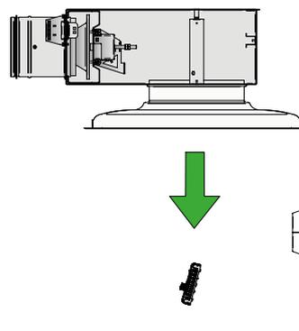
Figure 7. Replacement of WISE CU. Reassemble, in the reverse order and connect hoses and contactors from WISE CU, see "Connection". Apply the new supplied QR codes over the existing QR codes on the product.
