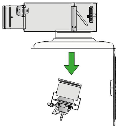
Figure 6. Dismantling the damper insert. Reassemble, in the reverse order.
