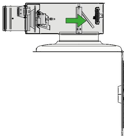
Disconnect the measuring tubes and damper motor cable.
