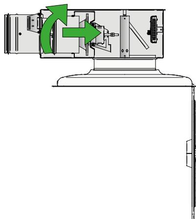
Turn the damper insert so that the bayonet fitting releases.
