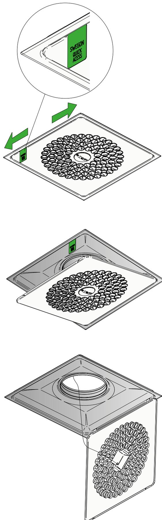
Figure 4. Suspension of WISE Colibri C, connection of WISE SMB.
