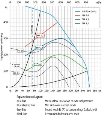
Recommended work area max SFP in relation to airflow and pressure
