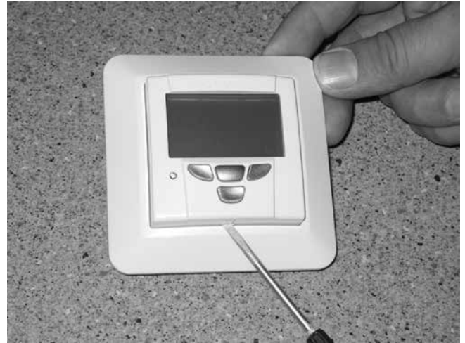
To dismantle the front plate on a Premium control panel.
