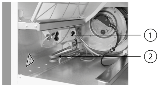
1. Overheat protection 2. Air reheater, overheating protection
