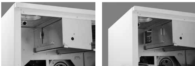
Bypass past the heat exchanger: The cover closed in the winter; open in the summer.
