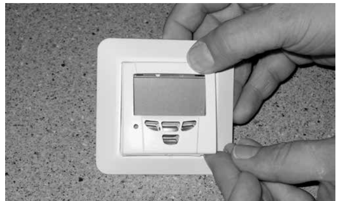
To secure the panel cover on the Premium control panel. First place the upper edge of the cover in place and then press the cover to secure it.
