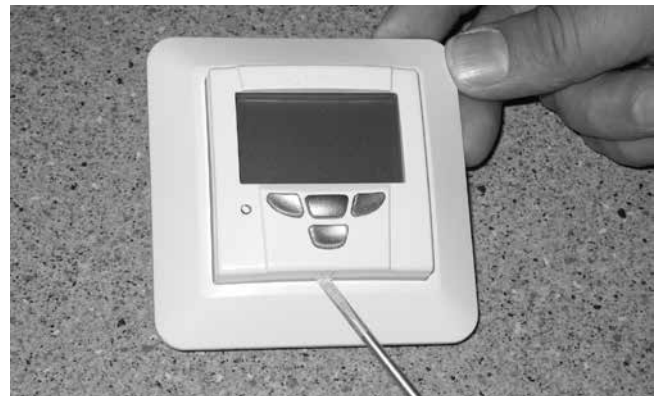
To dismantle the front plate on a Premium control panel.
