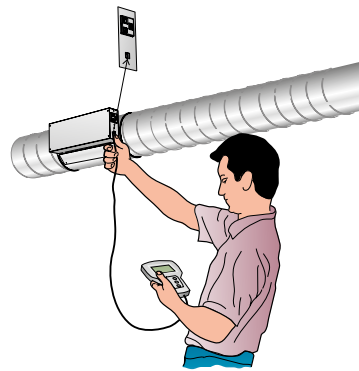
Figure 5. Wiring TUNE Adapt for checking and changing set points. Connection is made directly into the single socket on the side of the damper or the connection box of the extension cable. If DETECT SME is installed, TUNE Adapt is connected to SME instead. Communication with the parent system is disconnected while TUNE Adapt is connected.
