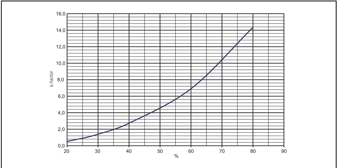
**Graph 1.** k-factor graph. k-factor for the different sizes of terminals and damper position in %.
