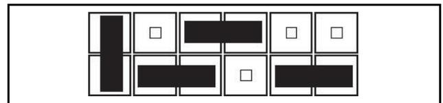
**Figure 3.** Shows the jumper positions for on/off control of the heating on output 4.
