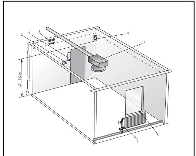
**Figure.** The components normal location.
