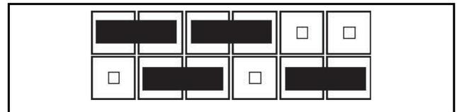
**Figure 2.** Shows the standard jumper positions for use in the e.r.i.c. System and for the VAR.
