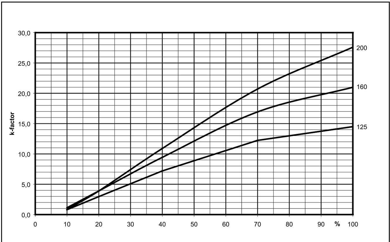
**Graph 2.** k-factor graph ACLb (as from 1 January 2006). k-factor for the different sizes of terminals and damper position in %.
