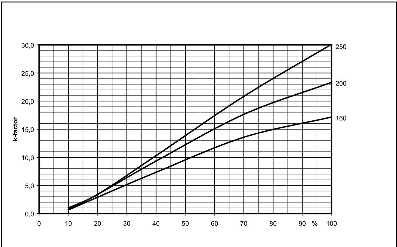
**Graph 2.** k-factor graph ACKc (as from 1 January, 2006). k-factor for the different sizes of terminals and damper position in %.
