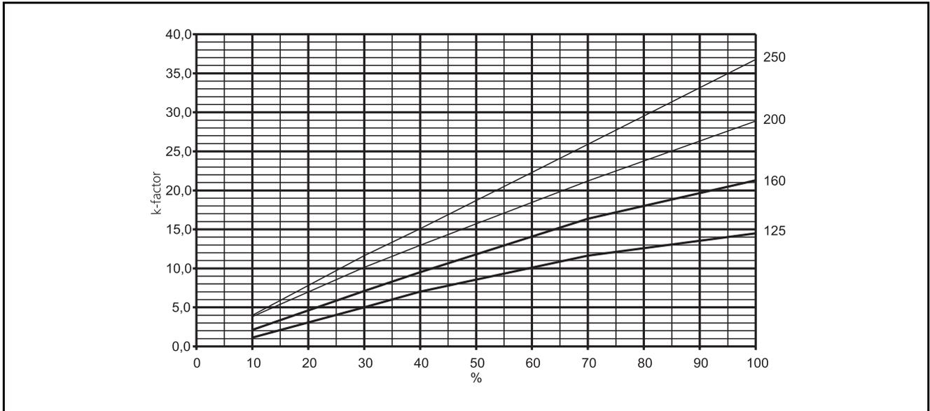
**Graph 1.** k-factor graph ACLa (before 31 Dec. 2005). k-factor for the different sizes of terminals and damper position in %.
