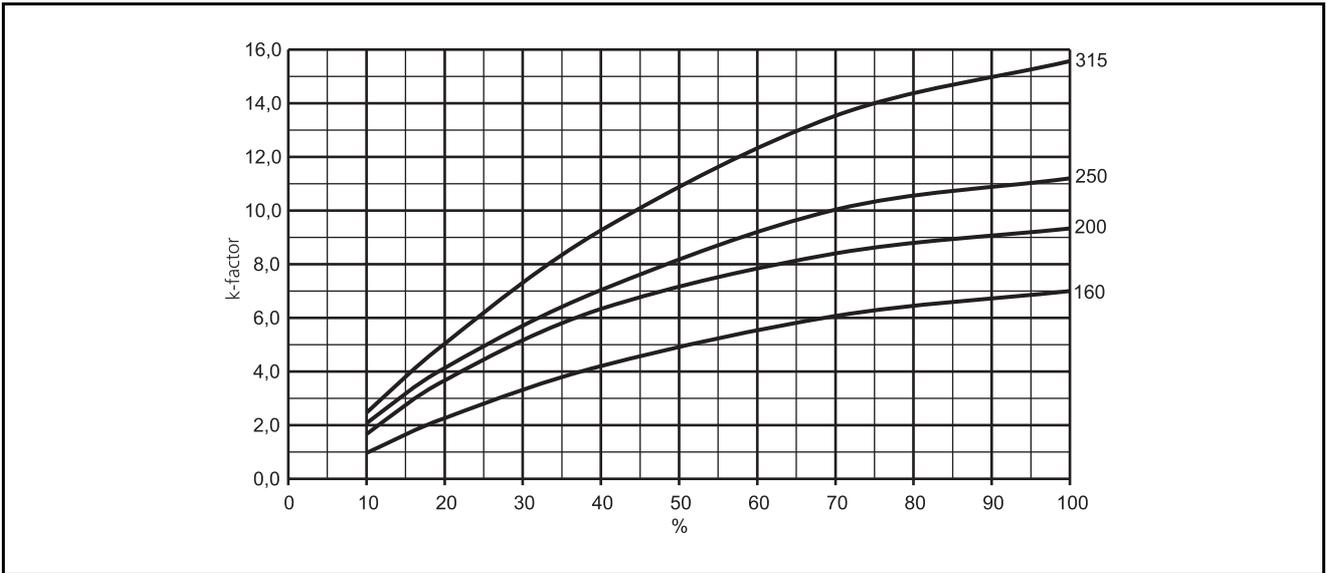
**Graph 1.** k-factor graph AFKb (before 31 Dec. 2005). k-factor for the different sizes of terminals and damper position in %.
