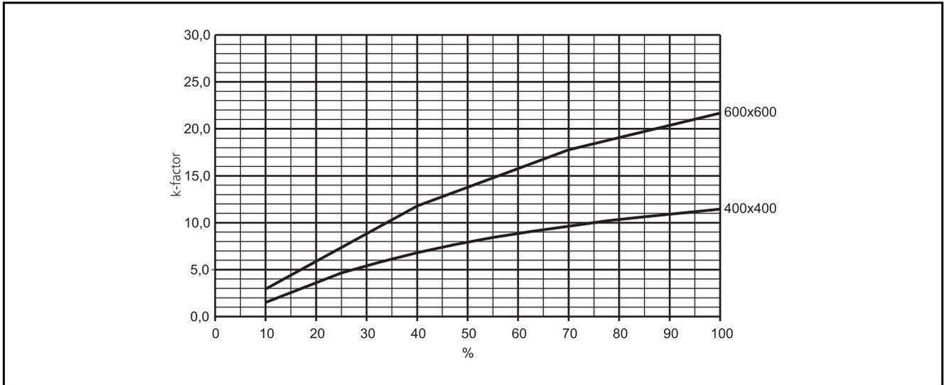
**Graph 1.** k-factor graph AKYb (before 31 Dec. 2005). k-factor for the different sizes of terminals and damper position in %.
