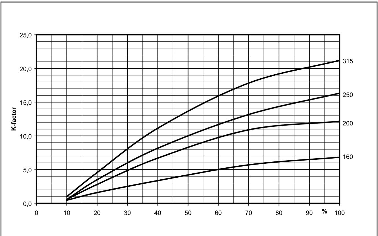
**Graph 2.** k-factor graph AFKb (as from 1 January 2006). k-factor for the different sizes of terminals and damper position in %.
