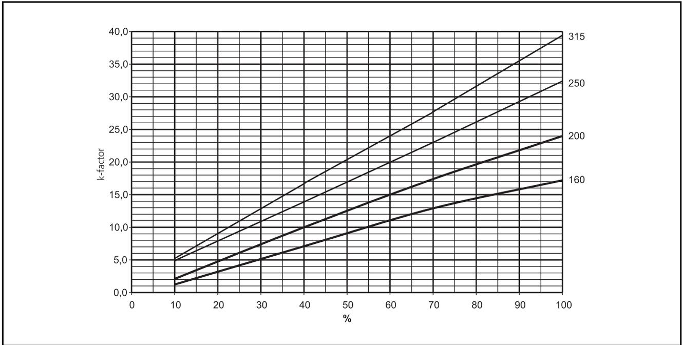
**Graph 1.** k-factor graph ACKb (before 31 Dec. 2005). k-factor for the different sizes of terminals and damper position in %.
