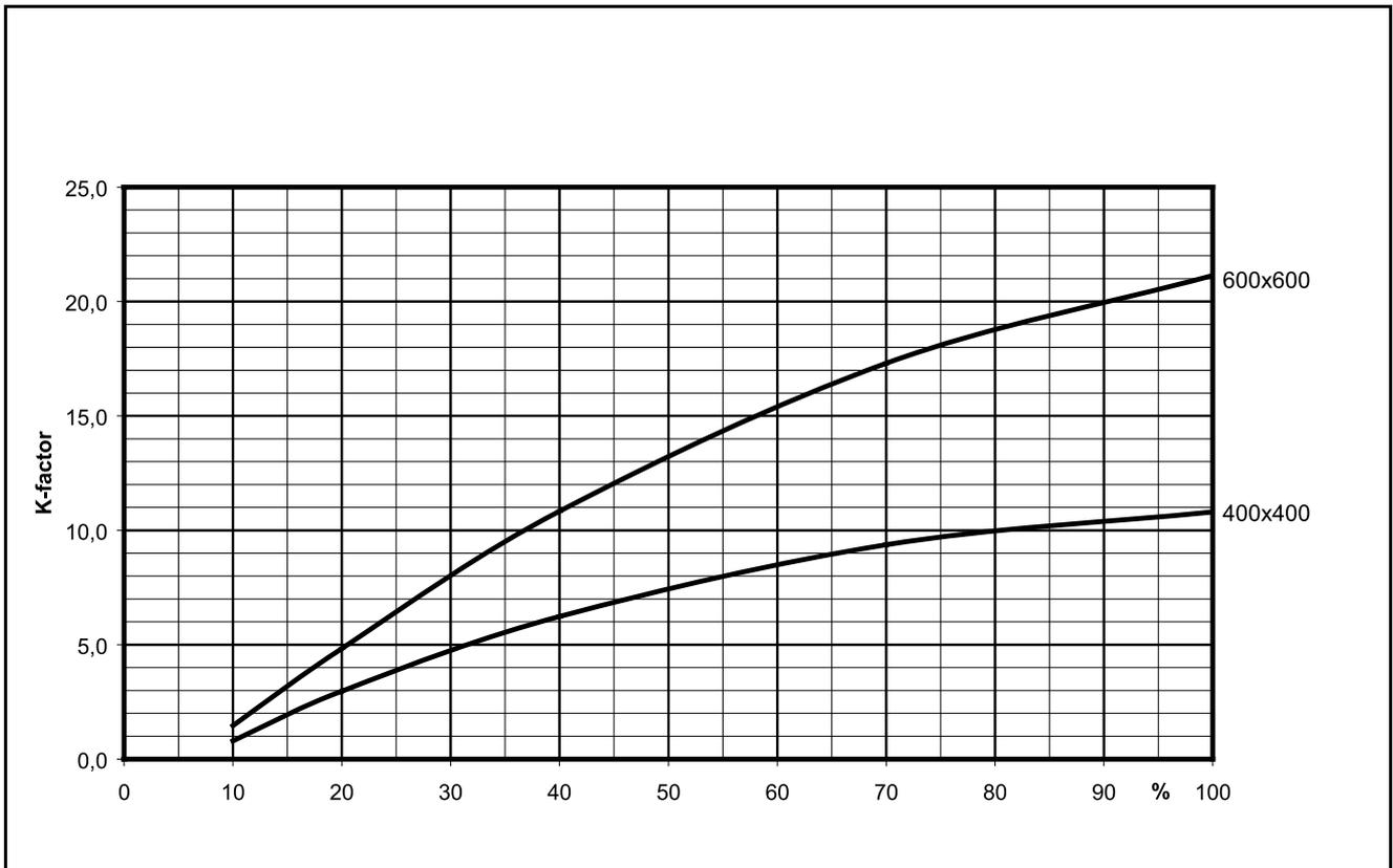
**Graph 2.** k-factor graph AKYb (as from 1 January, 2006). k-factor for the different sizes of terminals and damper position in %.
