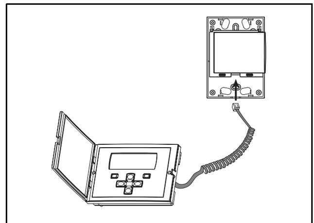
**Figure 2.** Connection of the terminal KOP to products with room unit KRF, KCD and KCW. KOP connects to on the inside (KSTb). The older KSTa connects to on the underside. In some executions on the side of the regulator casing.
