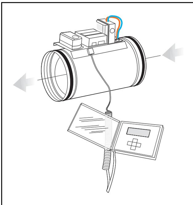
**Figure 1.** Connection of the hand terminal KOP to duct the products KZP, KZM, KSA and KRF.
