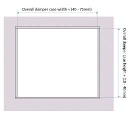
3. Calculate the hole to cut size by adding two board thicknesses to the finished hole width and height...
