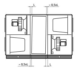
The illustration shows an appropriate rotor inclination setting for Fan Arrangement 1. The inclination must always be toward the filter, which means that the inclination for Fan Arrangement 2 is in the other direction.
