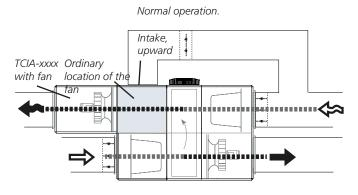
Solution for fire bypass (upward) for GOLD PX 04-08.
