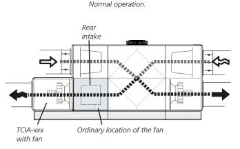
Solution for fire bypass (rear) for GOLD PX 04-08.
