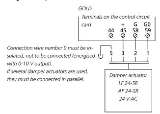
Under normal operating conditions, the damper opens and closes by means of the damper actuator's motor drive (actuating time: 90 seconds).
