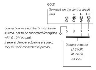
Under normal operating conditions, the damper opens and closes by means of the damper actuator's motor drive (actuating time: 90 seconds).
