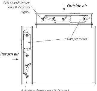
Fully open damper on a 0 V control signal. The direction of travel of the damper actuator must be changed. See Item 6.
