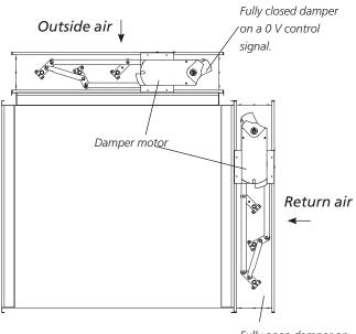
Fully open damper on a 0 V control signal.
