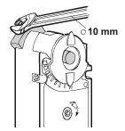
2. Remove the damper actuator from the damper spindle. It might be necessary to also remove the lower bracket.
