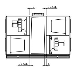
The illustration shows the factory-preset rotor inclination for Fan Arrangement 1. The inclination must always be toward the filter, which means that the inclination for Fan Arrangement 2 is in the other direction.
