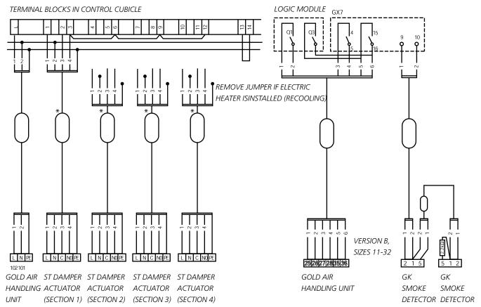
IF MORE SMOKE DAMPER ACTUATORS ARE INSTALLED, THEY SHOULD BE CONNECTED IN PARALLEL AT THE JUNCTION BOX.
