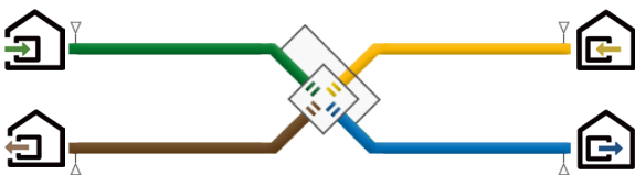
Plate heat exchanger
