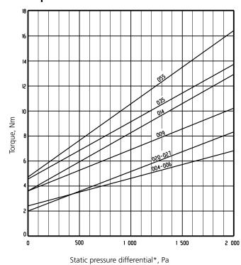
The size 004–014 mixing sections are equipped with three dampers. These three dampers are interconnected, which means that only one actuator is required. The torque has been calculated for all three dampers.
