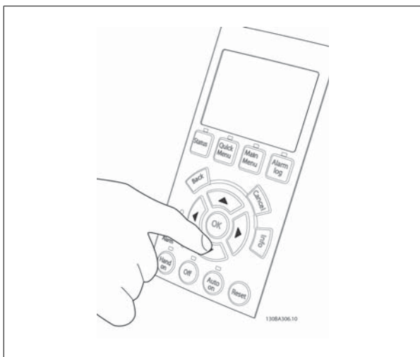
Illustration 4.42: Step 7: To move the cursor, use the left ◀ and right ▶ arrow buttons. This enables changing the speed in larger increments.
