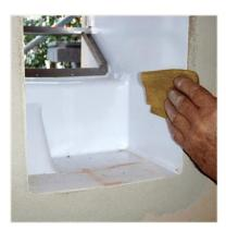
3. Support the appliance with your right hand in front and bottom and slide it straight into the box. Slide by pressing the front panel on the unit until it stops.
