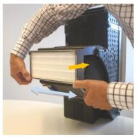
3. Pull the extract filter out of the side of the device and insert a new original bluMartin-filter in the correct direction (note the arrow AIR FLOW).
