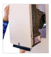
6. To reset the filter hour counter shortly change into Service mode. To do that turn first the device off (wait till all LEDs are off).
