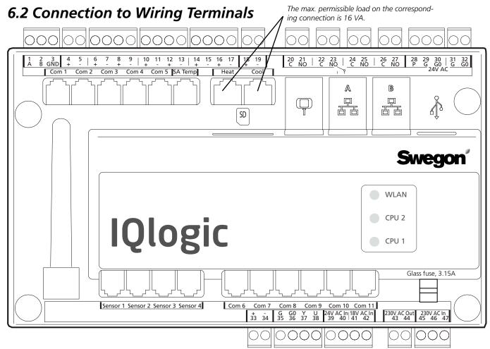
Digital inputs, terminals 4-17, are of extra-low voltage type. Analogue input, terminals 18-19 have an input impedance of 66  $k\Omega$ . 230 VAC control voltage is on external terminals 101 (L) and 102 (N).
