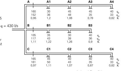
qp = design airflow (l/s)gm = flow reading (l/s)
