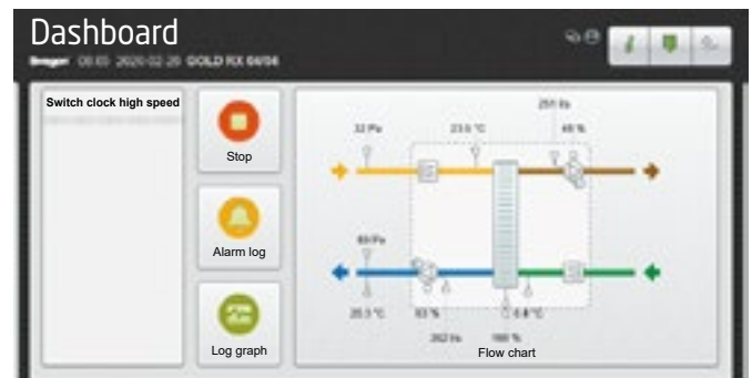
Example of a flow chart from the built-in web server.
