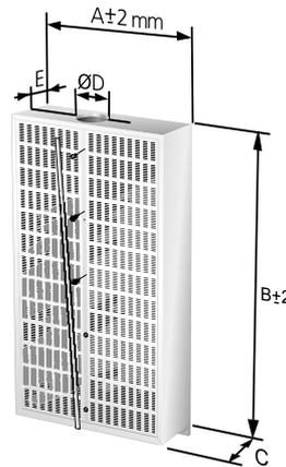
Figure 7. Maintenance for two-piece front with  $A=1190$  mm and circular connection, dismantle the cover strip and then the screws that secure the front plate, lift and pull out.
