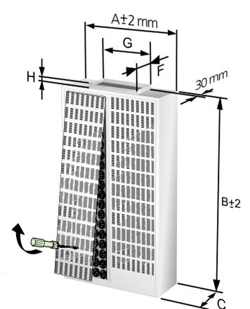
Figure 8. Maintenance for two-piece front with  $A=1190$  mm and rectangular connection, dismantle the cover strip and then the screws that secure the front plate, lift and pull out.
