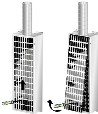
Figure 6. Maintenance for one-piece front with  $A=590$  mm and circular connection 200 and 250, lift and pull out.
