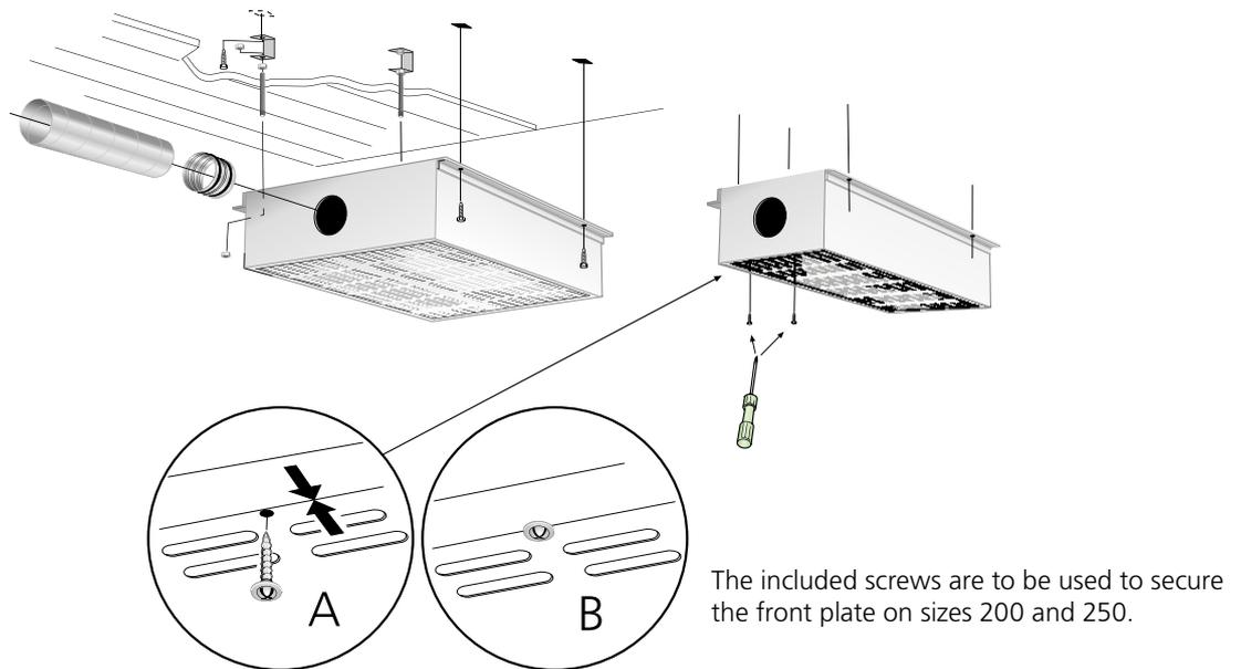
Figure 1. Installation ceiling.
