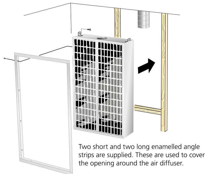
Figure 3. Recessed installation.
