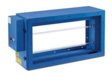
TRION $_{\odot}$  Saber UV deodorization equipment, uses the ultraviolet light generated by the UV lamp and ozone generated in the reaction of oxygen in the air, photolysis oxidative decomposition of odour in smoke and oil, thereby effectively reducing the odour in the exhaust. Suitable for places where odours of food fumes are purified, such as restaurants, hotels, commercial building restaurants, food courts and etc.
