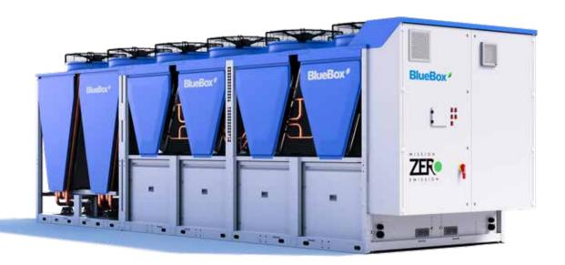
Double circuit Free-cooling chillers featuring reciprocating semi-hermetic inverter compressors and R290 natural refrigerant. Free cooling coil with independent modular design.
