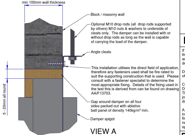
The penetration seal is to be finished with an ablative coating that is compatible with the make of Fire Batt used. Please refer to the specific ablative coating instruction for guidance on application.
