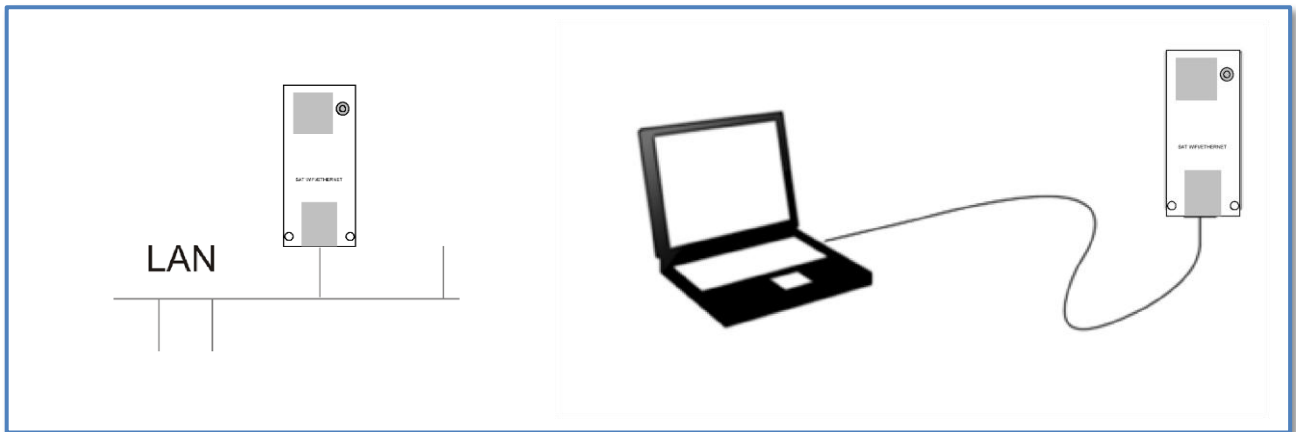
Figure 3 - SAT WIFI-ETHERNET connection in a LAN
