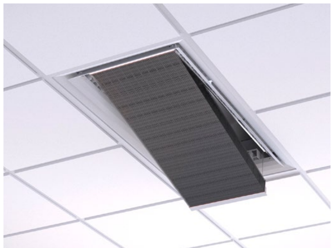
Figure 11. Removing the face plate and folding out the coil for accurate cleaning in the event of high hygiene requirements. Note! requires the product to be ordered with the accessory fold-out coil, and that flexible connection hoses are used on the water side.
