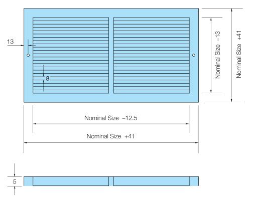
Grilles supplied with screw hole in flange as standard.
