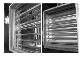
The louver damper positioner can be mounted on the interior, as well as on the exterior of the housing. It should be mounted on the interior of those units designed for outside use, or protected against moisture.
