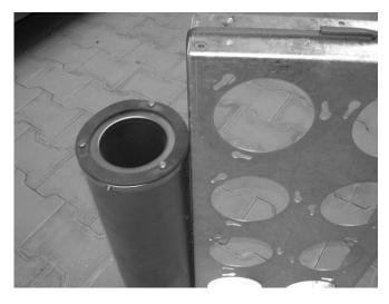
In order to ensure a fault-free functioning of the filter cartridge, an odour check following filtering should be carried out. If necessary, the cartridge should be replaced.
