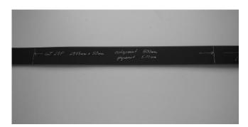
It must be heeded that the belt tension is checked after the first 100 operating hours, and re-tensioned as necessary.
