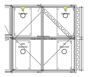
Here too, after installation, the joints between the plate heat exchanger and housing must be sealed with sealant.
