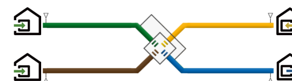
Plate heat exchanger
