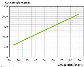
Diagram a. Example: 25% CAC output signal is equivalent to CO<sub>2</sub> 800 ppm.
