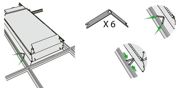
Figure 20. Kit de centrage SYST CENTERING KIT PARASOL
