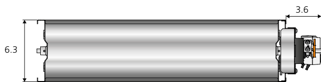
Figure 8. Dimensions (in), REACT P GMB rectangular.
