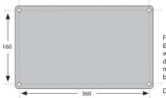
Four mounting holes Ø 6mm for mounting with suitable screws depending on whether mounting to a duct, block wall or stud wall.
