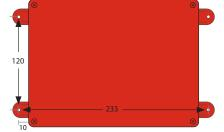
Four mounting holes Ø 6mm for mounting with suitable screws depending on whether mounting to a duct, block wall or stud wall.
