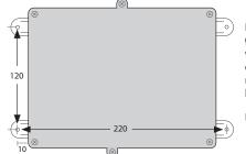
Four mounting holes Ø 6mm for mounting with suitable screws depending on whether mounting to a duct, block wall or stud wall.
