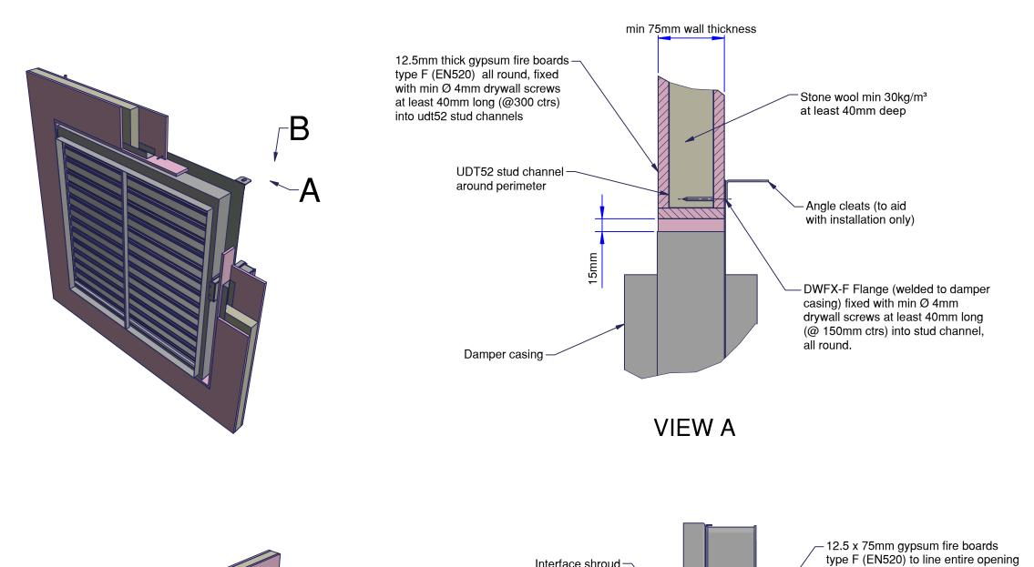
DWFX-F Flange (welded to damper casing) fixed with min Ø 4mm drywall screws at least 40mm long (@ 150mm ctrs) into stud channel,
