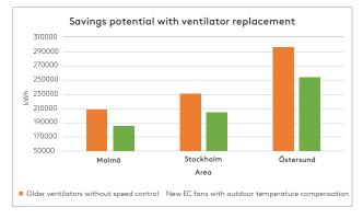
The bars show the energy consumption for an older (25-30 years) AC fan without speed control, compared to a newly installed EC fan with the outdoor temperature compensation function activated for three locations in Sweden
