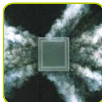
Irregular air distribution
