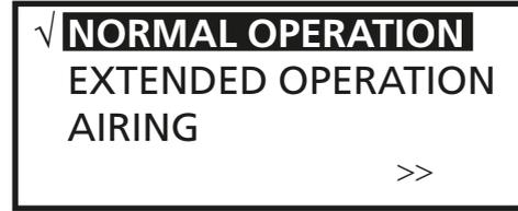
If the room is to be used one evening, for instance, and the timer then has controlled the air handling unit to operate at low speed, you can activate the EXTENDED OPERATION function. The fans in the air handling unit will then operate at high speed during the preset period (Factory Setting: 45 minutes).
