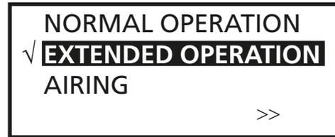
If many people occupy the room at the same time, for instance, you can activate the AIRING function (preferably during a pause). The fans in the air handling unit will then operate at high speed during the preset period (Factory Setting: 15 minutes) and thus try to reach a preset supply air temperature.
