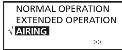
When the preset period for EXTENDED OPERATION and AIRING has expired, the COMPACT Air unit will automatically return to normal operation.
