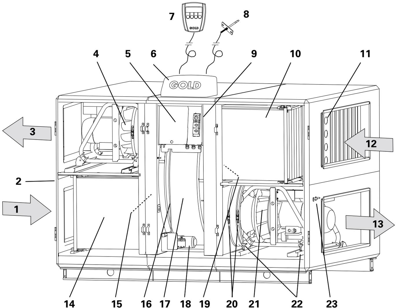
The air handling unit is supplied as a right-hand unit, i.e. with the airflow directions indicated by the arrows in the illustration. If you alter the installation to obtain a left-hand flow configuration, the components marked with an asterisk exchange function and name (i.e. they must be renamed accordingly if their function is for supply air or for exhaust air).
