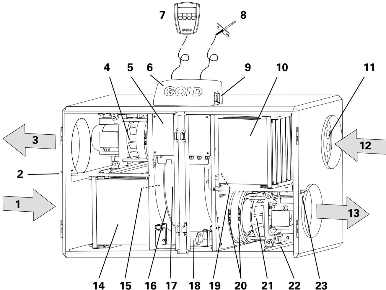
The air handling unit is supplied as a right-hand unit, i.e. with the airflow directions indicated by the arrows in the illustration. If you alter the installation to obtain a left-hand flow configuration, the components marked with an asterisk exchange function and name (i.e. they must be renamed accordingly if their function is for supply air or for exhaust air).
