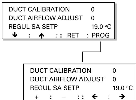
DUCT CALIBRATION is normally set at 0 (off). If duct calibration is activated (1=on), the unit will run at a fixed calibration speed and the controller will measure where in the flow chart the unit is operating with regard to connected duct system. Duct calibration provides the reference for the alarm limit used in the filter tests. The unit must therefore have clean filters when duct calibration is begun.
