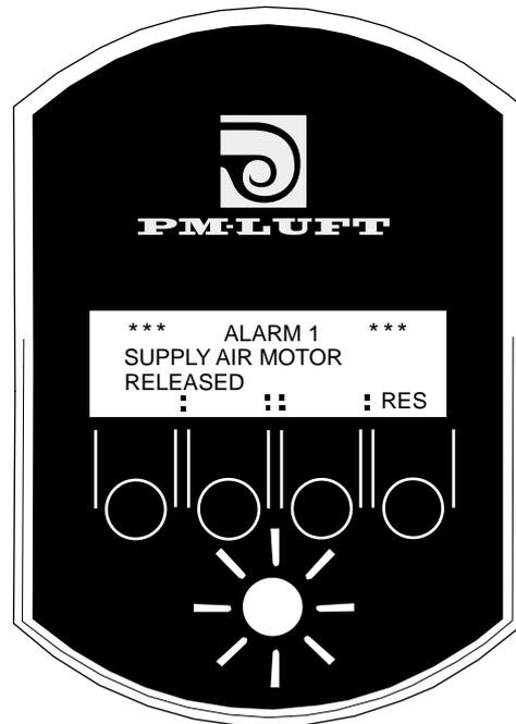
*The control display with flashing alarm lamp.*
