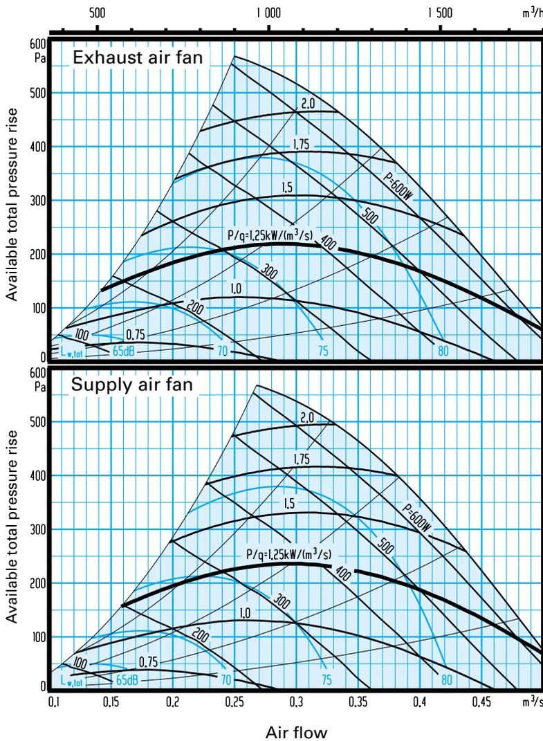
The sizing chart shows the min. and max. available total pressure rise required to cover the pressure drop in the ducting in relation to:
