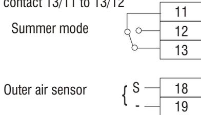
The temperature sensor must be installed in the outside air. When ordering, this function is indicated by the letter "D" (see page titled "Ordering controllers").
