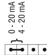
For a control signal of 0 - 10 V, the pins must be jumped as illustrated below.
